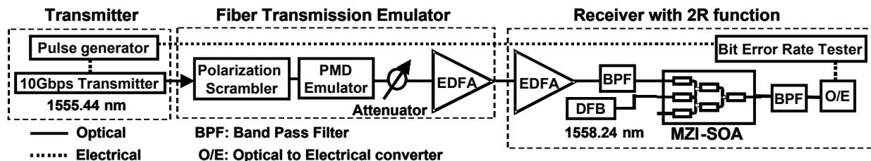
Figure 1: Experimental setup of PMD margin generation by MZI-SOA
