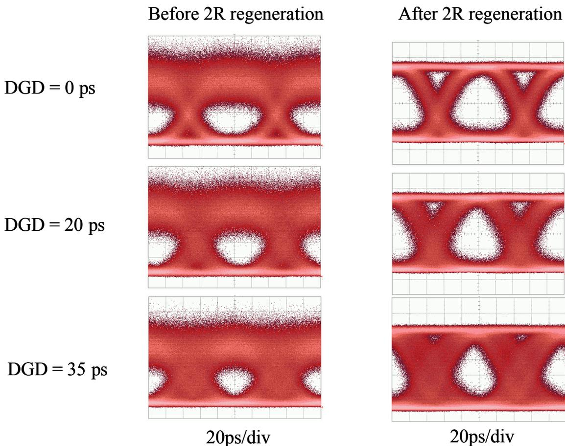
Figure 2: Eye diagrams before and after 2R regeneration with 0, 20 or 35ps DGD (18dB OSNR/0.1nm)
