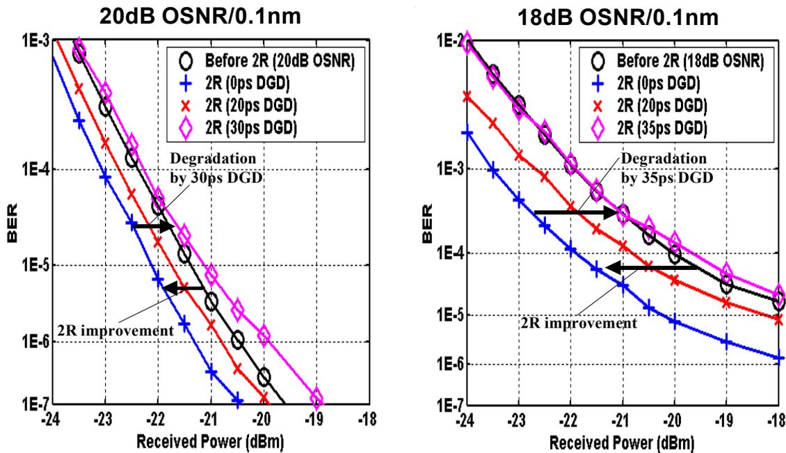
Figure 3: BER curves of 2R regeneration with 0, 20, 30 or 35ps DGD (Left: 20dB OSNR/0.1nm, Right: 18dB OSNR/0.1nm)
