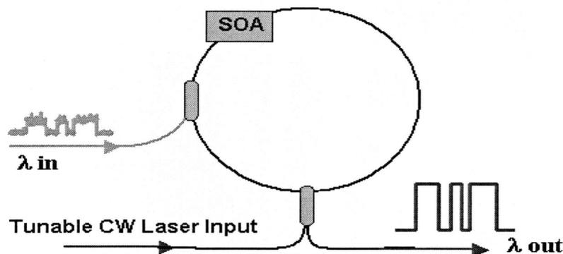
Fig.1. Schematic diagram of the tunable all-optical signal regenerator (TASR)
