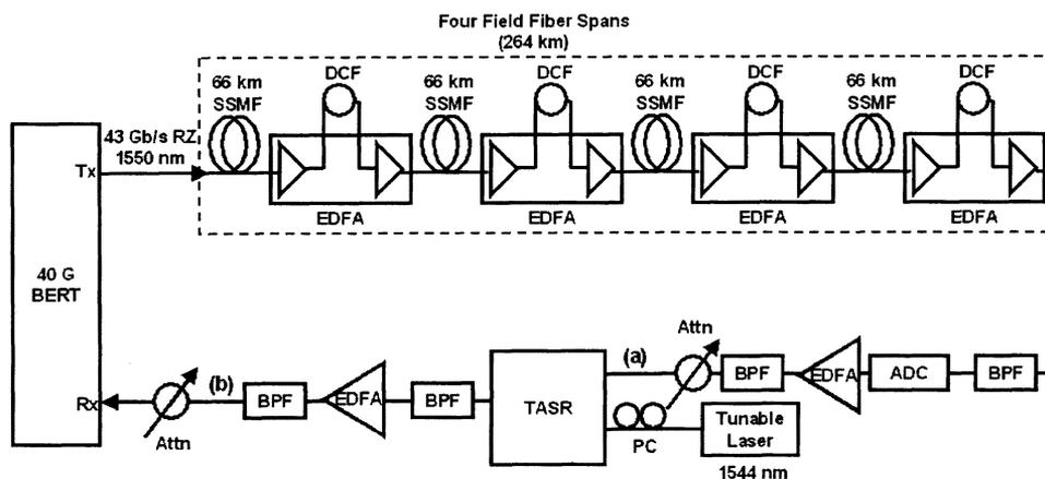
Fig. 2. Experimental setup. BERT: Bit Error Rate Tester; Tx: Optical Transmitter; Rx: Optical Receiver; SSMF: Standard Single-mode fiber; DCF: Dispersion Compensating Fiber; BPF: Optical Tunable Band-pass Filter; ADC: Adaptive Dispersion Compensator; EDFA: Erbium Doped Fiber Amplifier; Attn: Optical Variable Attenuator; PC: Polarization Controller; TASR: Tunable All-optical Signal Regenerator.
