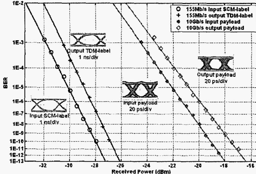
Fig. 4. BER measurement results for the label and the payload before and after the labeling format conversion operation
