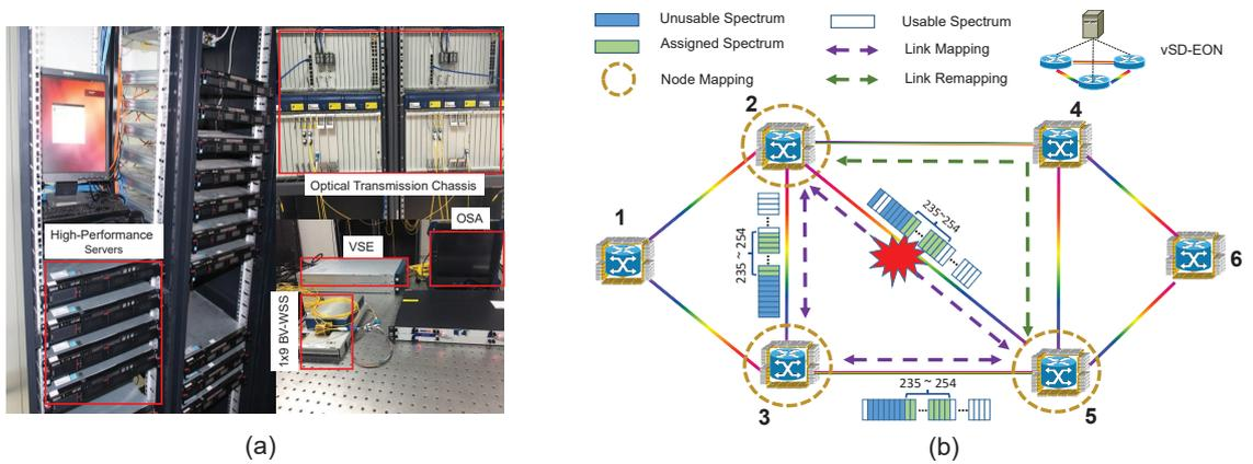
Fig. 2. (a) Experimental testbed, VSE: video streaming equipment, OSA: optical spectrum analyzer; and (b) Substrate topology and the vSD-EON to be embedded.
