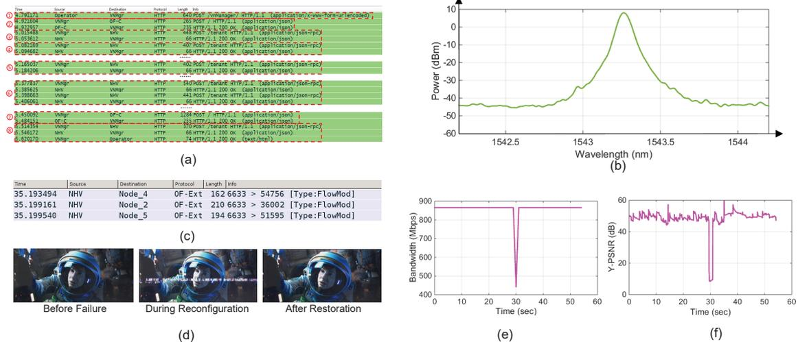
Fig. 3. (a) Messages used for vSD-EON creation, (b) Optical spectrum of the virtual lightpath, (c) Messages used for VL remapping, (d) Screen-shots of video playback, (e) Throughput of video streaming, and (f) PSNR of video playback.
