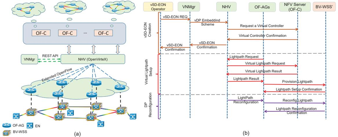
Fig. 1. (a) Architecture of our vSD-EON slicing system, EN: end-node; and (b) Operation procedure for 1) vSD-EON creation, 2) virtual lightpath setup, and 3) DP restoration with lightpath reconfiguration (*i.e.*, virtual link remapping).
