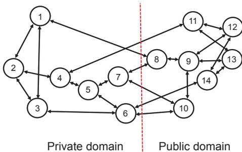
Fig. 4. MD-EON derived from the NSFNET topology.
