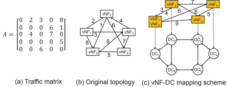
Fig. 3. Example on the vNF-DC mapping scheme.
