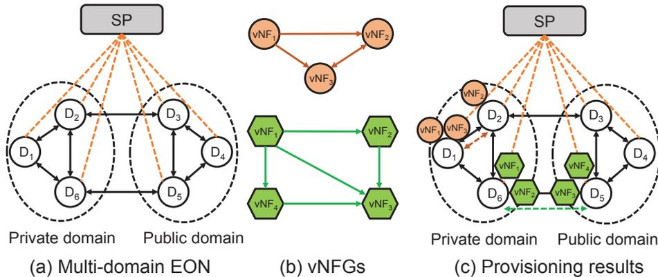
Fig. 1. Example on provisioning vNFGs in an MD-EON.
