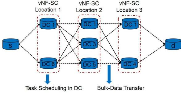
Fig. 2. Example of constructing auxiliary graph in the proposed DP-based algorithm.
