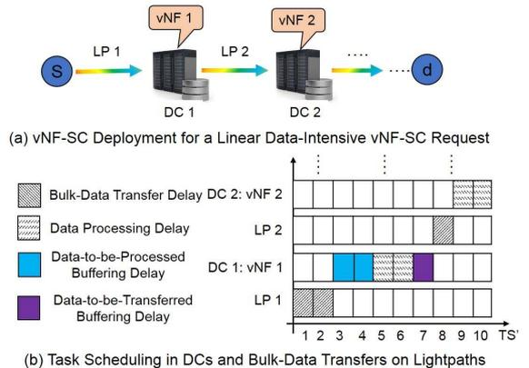
Fig. 1. Example of vNF-SC deployment and traffic steering for a linear data-intensive vNF-SC request.
