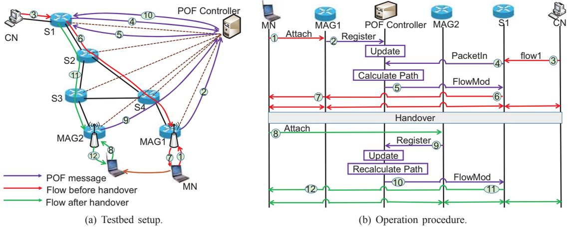
Fig. 5. Experimental demonstration of POF-SR based mobile management.
