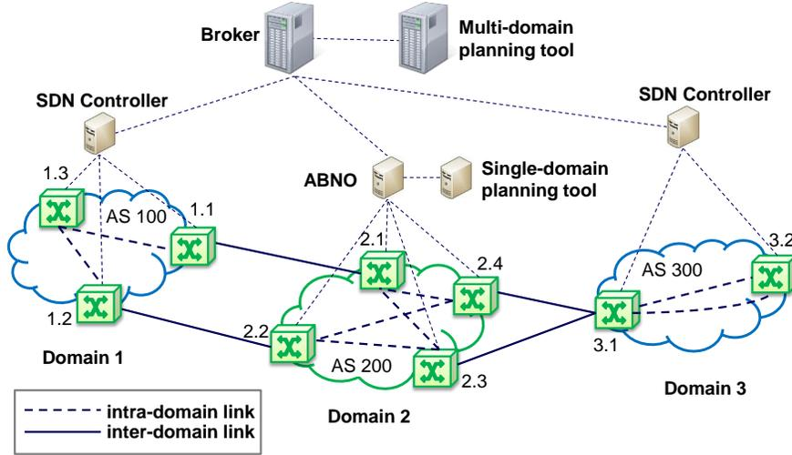
Fig. 1. Multi-AS network architecture.
