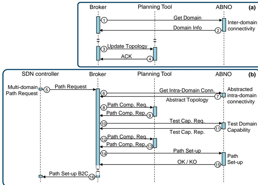
Fig. 3. Proposed workflows. a) Domain advertisement and b) Path computation and set-up.
