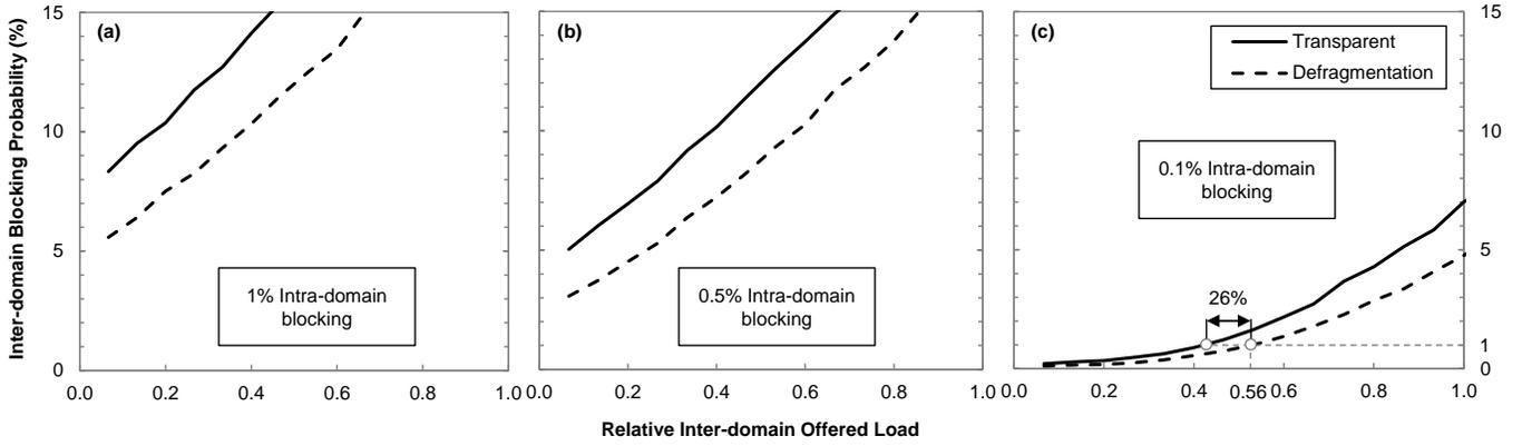
Fig. 6. Inter-domain blocking probability against relative intra-domain offered load, when domains are loaded so the resulting intra-domain blocking probability is (a) 1%, (b) 0.5%, and (c) 0.1%.
