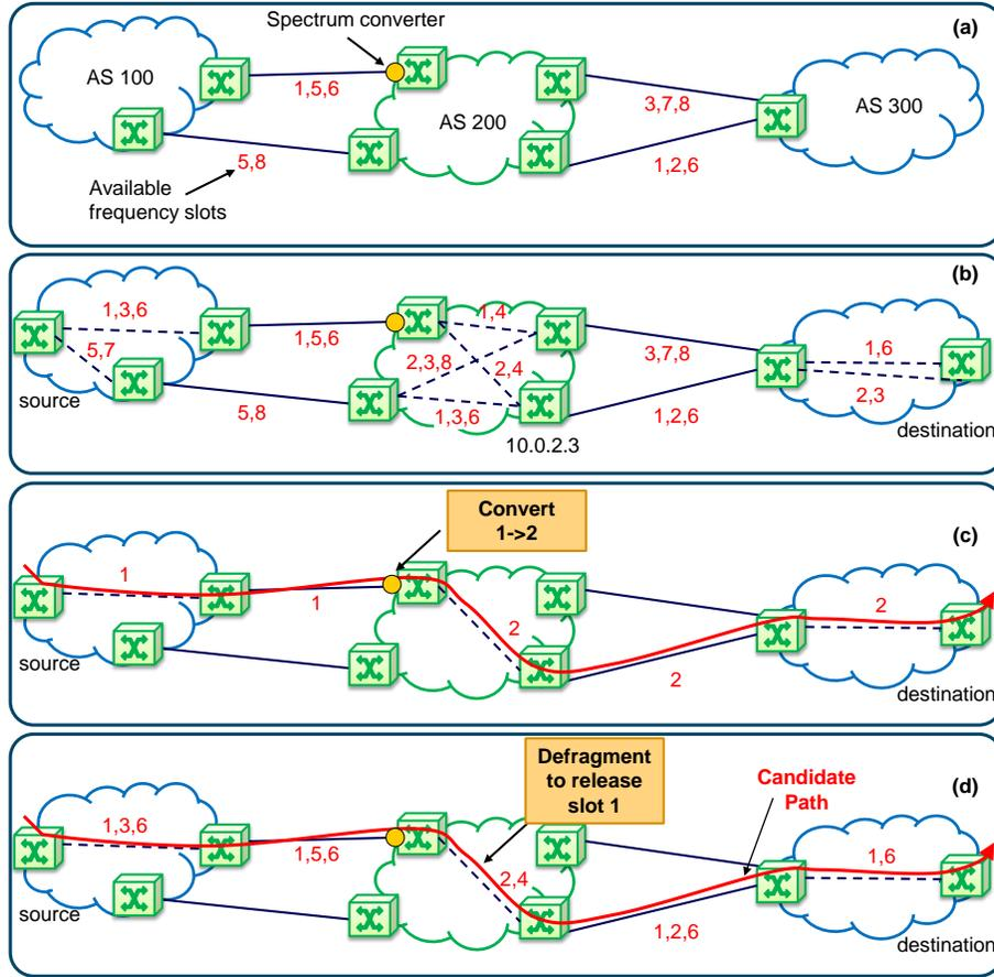
Fig. 2. An example of path computation. a) Initial AS advertisement and inter-AS link updating. b) Abstracted intra-AS and end-nodes advertisement. c) Path computation using the conversion capability. d) Path computation using the defragmentation capabilities.
