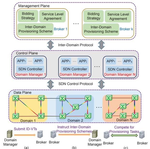
Fig. 1. Network architecture of a multi-broker based multi-domain SD-EON, and the actions (a) from domain managers to brokers, (b) from brokers to domain managers and (c) among brokers.
