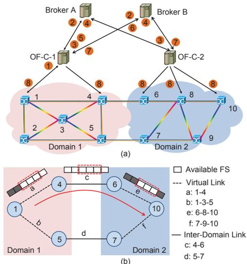
Fig. 3. Operation principle of multi-broker based multi-domain SD-EON system, (a) working procedure and (b) ID-VT abstraction.
