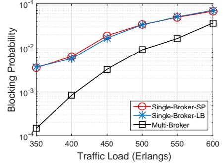
Fig. 8. Request blocking probabilities from single- and multi-broker based scenarios.
