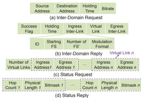
Fig. 4. Messages designed for the inter-domain protocol (IDP).
