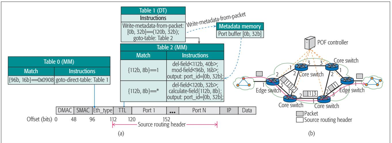
FIGURE 4. POF-based source routing: a) the procedure used to process the flow table in core switches and packet header designed for source routing; b) the operation principle of POF-based source routing.
