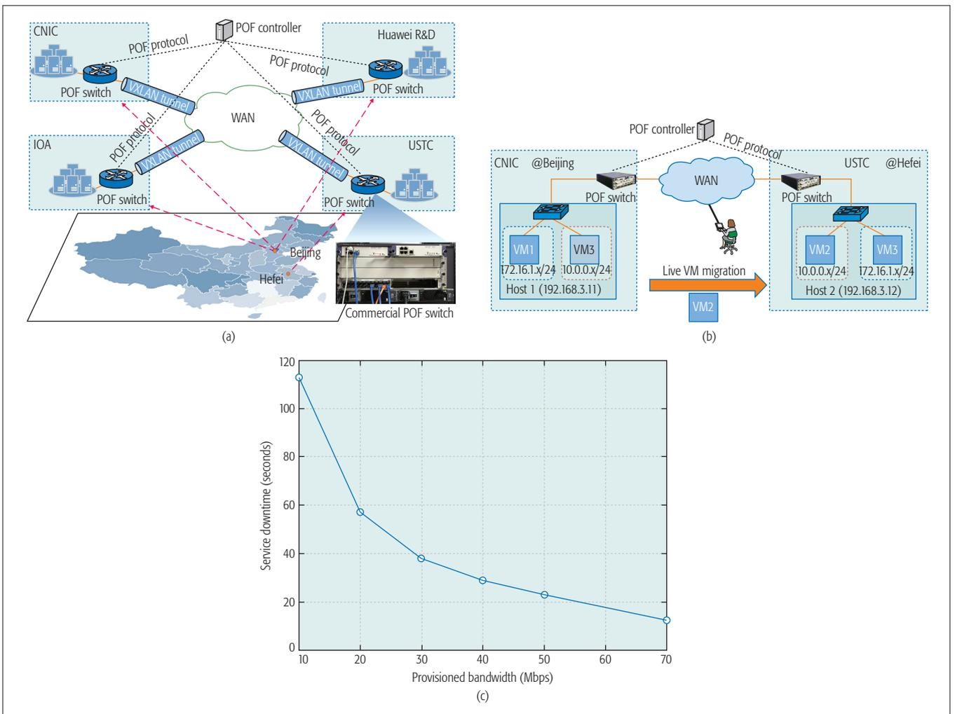
FIGURE 6. WAN-based POF network testbed in China: a) WAN-based POF network testbed in China; b) VM migration across WAN in POF network testbed; c) results on service downtime due to VM migration across WAN.
