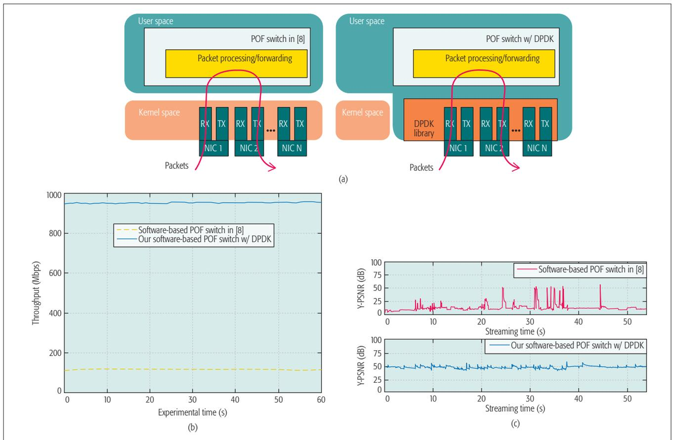
FIGURE 3. Design and performance of our software-based POF switch: a) architecture of our software-based POF switch with Intel DPDK; b) throughput comparison of software-based POF switches; and c) comparison on the Y-PSNR of received videos from different software-based POF switches.
