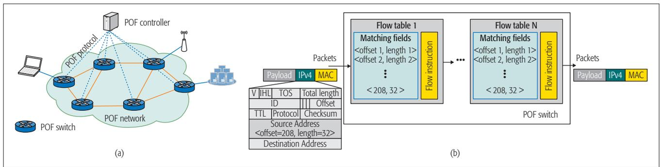
FIGURE 1. Overview of POF: a) architecture of a POF-based network; b) packet forwarding procedure in POF.
