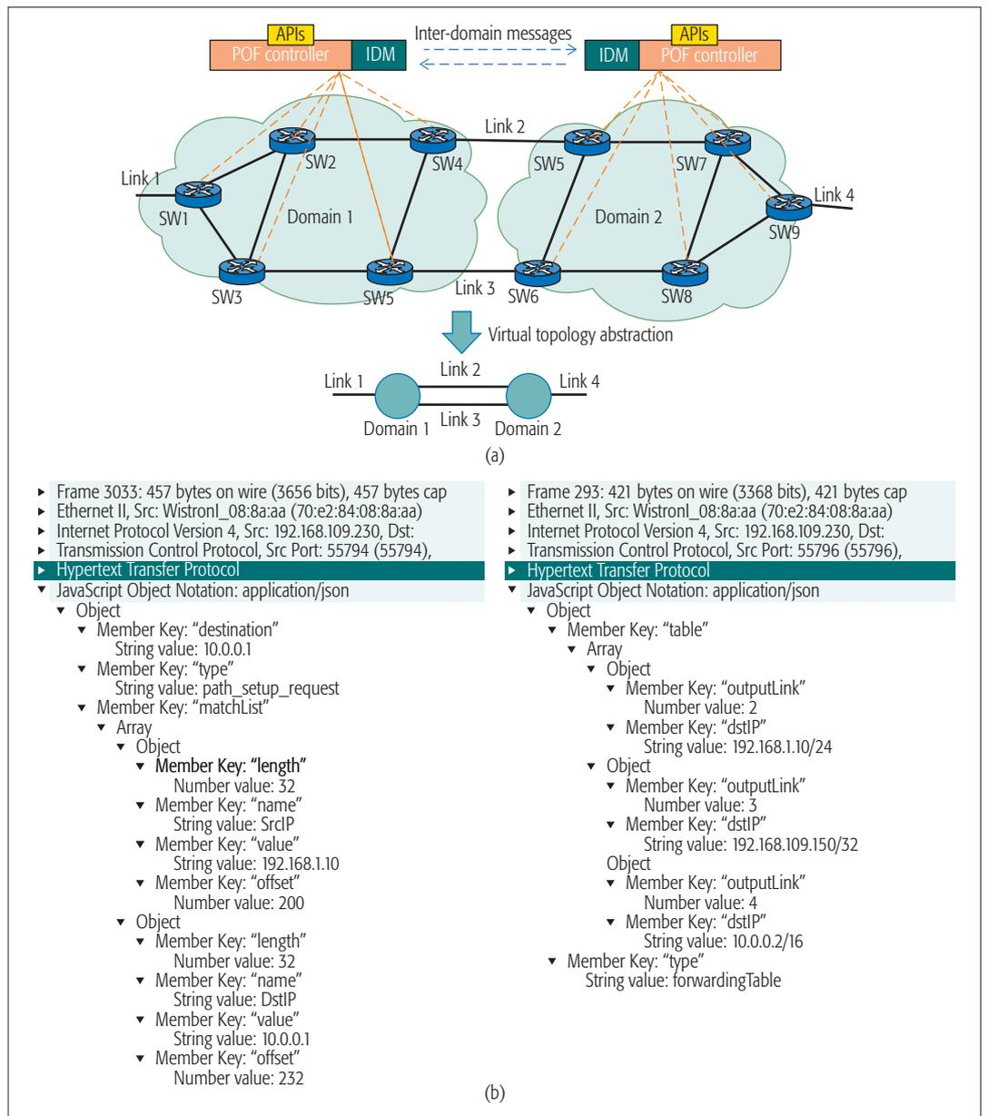
FIGURE 2. POF control plane for multi-domain scenarios: a) POF inter-domain operation; b) Wireshark captures of control packets to/from IDMs in POF controllers.
