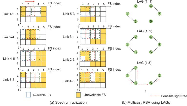
Fig. 2. Example on integrated multicast RSA using LAGs.
