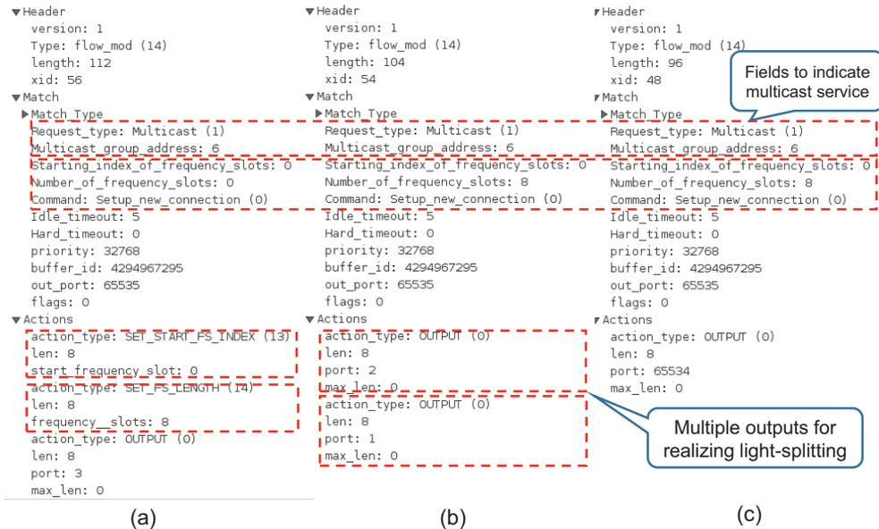
Fig. 9. FlowMod messages received by (a) the source node, (b) an intermediate light-splitting node, and (c) a destination node for setting up a light-tree.
