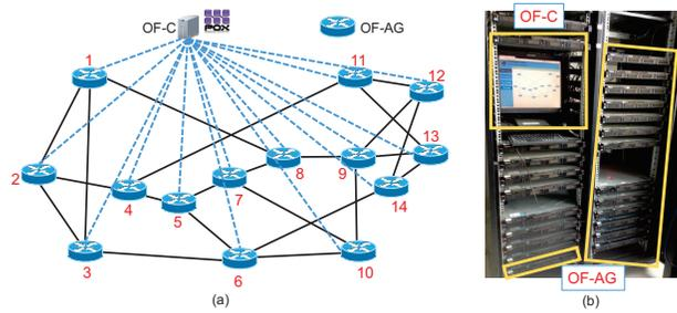
Fig. 6. Experimental setup: (a) control plane topology according to NSFNET, and (b) testbed built with high-performance servers.
