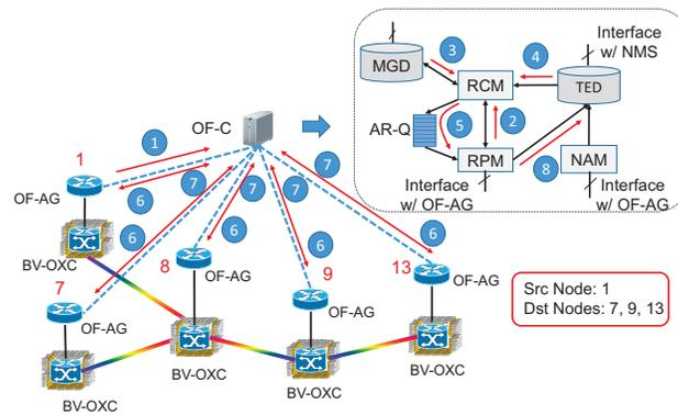
Fig. 7. Procedure for provisioning an AR multicast request (the blue circles contains step numbers).
