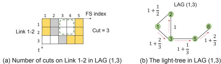
Fig. 4. Example of cut calculation and light-tree calculation
