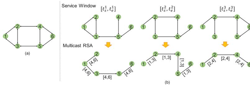
Fig. 1. (a) Six-node topology, and (b) Example on provisioning an AR multicast request.
