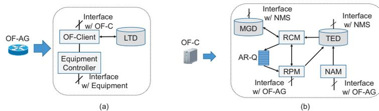
Fig. 5. Functional modules in (a) OF-AG and (b) OF-C.
