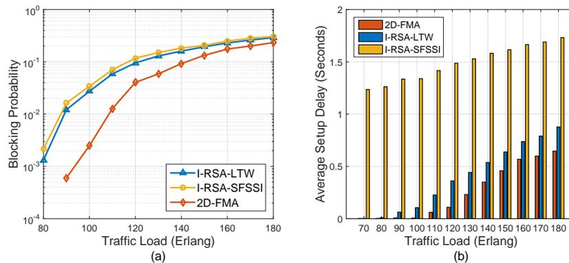
Fig. 10. Results on (a) request blocking probability and (b) average setup delay.
