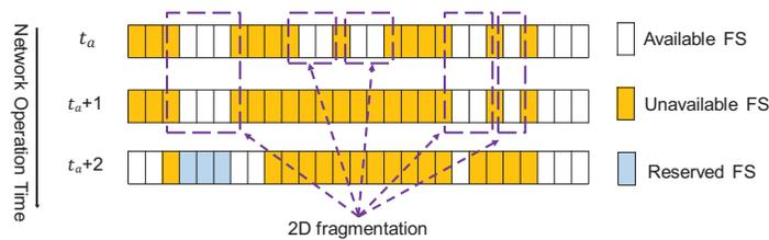
Fig. 3. Example for 2D fragmentation in an EON.
