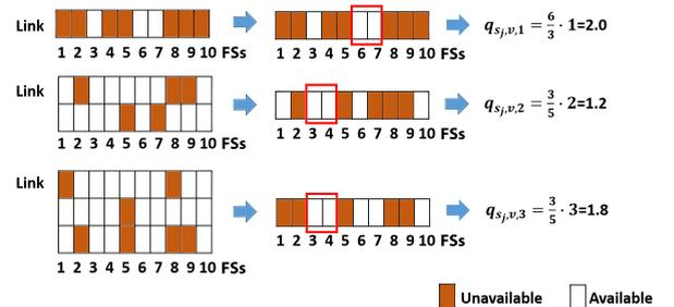
Fig. 2. Examples for calculating  $q_{s_j,v,k}$  in SUA-ITFRA.
