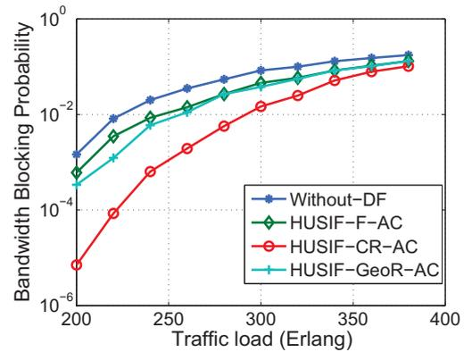
Fig. 4. BBP results of HUSIF based joint DF algorithms.
