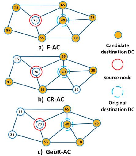
Fig. 2. Examples of destination selection in the anycast schemes.
