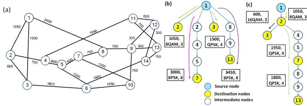
Fig. 1. (a) NSFNET topology (fiber lengths in kilometers). (b) An example of OL-Multicast. (c) An example of MOFR-Multicast.
