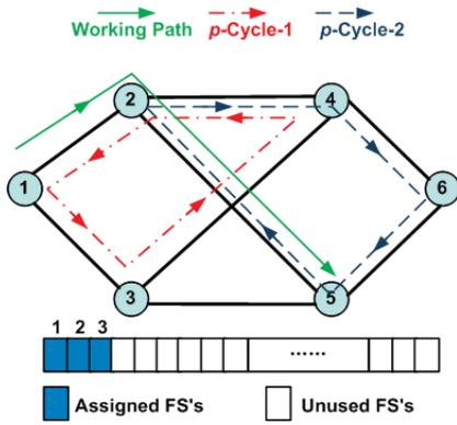
Fig. 1. An example of same-spectrum  $p$ -cycle protection in EONs.
