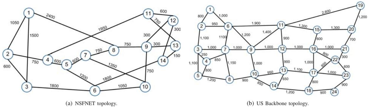
Fig. 4. The network topologies for the simulation (fiber lengths in kilometers).
