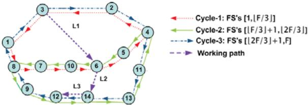
Fig. 3. An example of PWCE- $p$ -cycle-SP algorithm's drawback.
