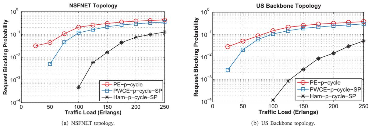
Fig. 5. Simulation results on request blocking probabilities.
