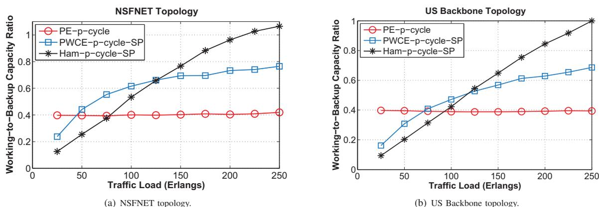
Fig. 6. Simulation results on working-to-protection capacity ratio.
