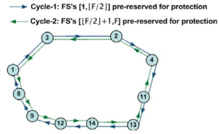
Fig. 2. An example of spectrum planning in PWCE- $p$ -cycle-SP.
