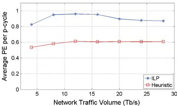
Fig. 6. Simulation results on average PE per *p*-cycle for static nonuniform traffic.
