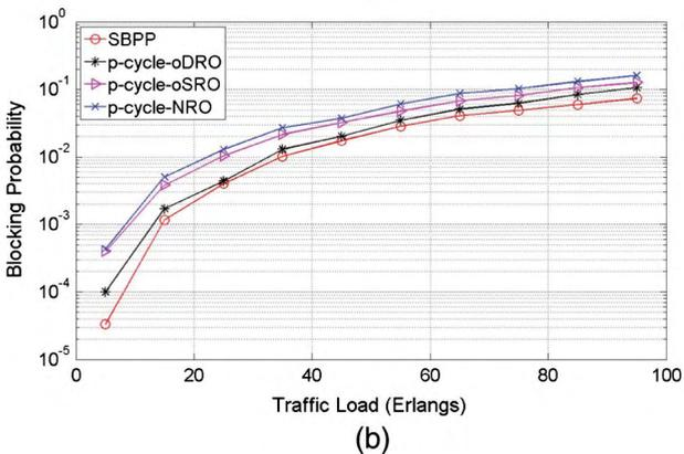
Fig. 8. Blocking probability versus traffic load from different dynamic resilience design algorithms: (a) Total energy budget is 15 k units and (b) total energy budget is 20 k units.
