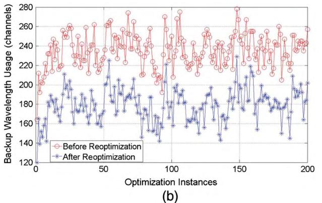
Fig. 9. Comparisons of (a) backup energy cost and (b) backup wavelength usage, before and after reoptimization with  $p$ -cycle-oSRO and the total energy budget of 15 k units.
