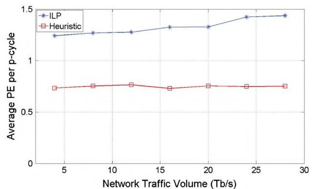
Fig. 4. Simulation results on average PE per  $p$ -cycle for static uniform traffic.
