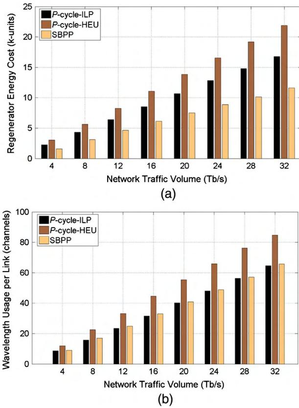
Fig. 5. Simulation results for static nonuniform traffic: (a) Total regenerator energy cost and (b) average wavelength usage per link.
