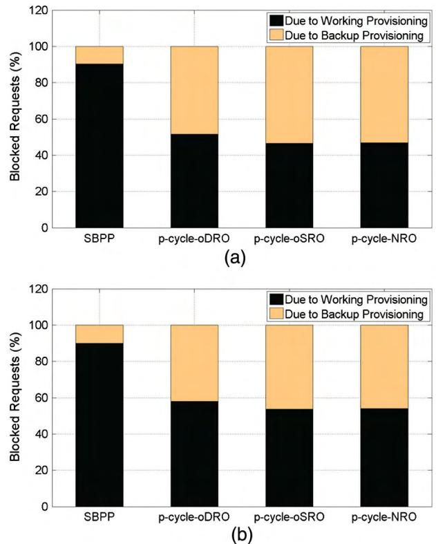
Fig. 10. Distributions of request blocking reasons for different dynamic resilience design algorithms: (a) Total energy budget is 15 k units and (b) total energy budget is 20 k units.
