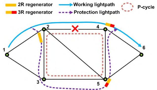
Fig. 1. Resilience based on a  $p$ -cycle in a translucent network with MRP.
