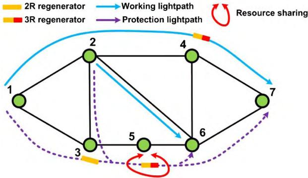
Fig. 7. Resilience based on SBPP in a translucent network with MRP.
