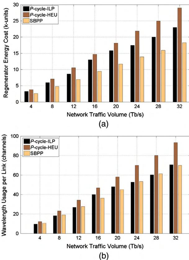
Fig. 3. Simulation results for static uniform traffic: (a) Total regenerator energy cost and (b) average wavelength usage per link.
