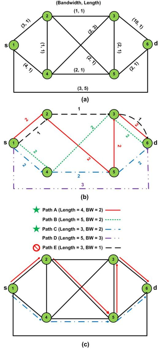
Fig. 1. Example of service provisioning using multipath routing with a BW-allocation granularity of  $g = 2$ . (a) Network topology  $G(V, E, B, D)$ . (b) Path computation results. (c) Elastic multipath provisioning scheme for a request with  $BW = 4$  and  $g = 2$ .
