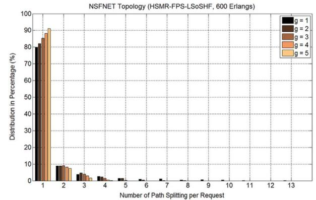
Fig. 9. Simulation results on the distribution of path splitting per request in NSFNET using the HSMR-FPS-LSoSHF scheme.
