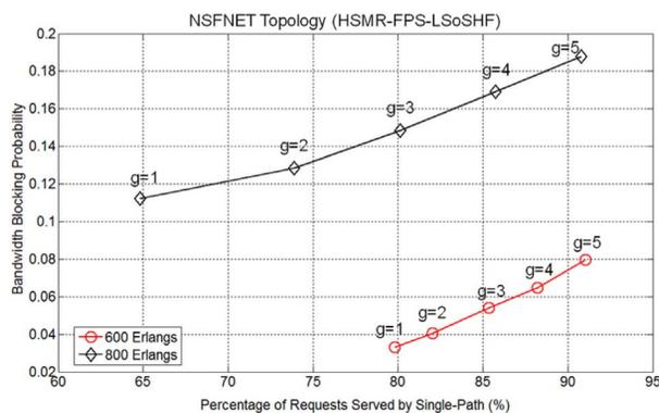
Fig. 10. BBP versus percentage of requests served by single-path in NSFNET using the HSMR-FPS-LSoS HF scheme.
