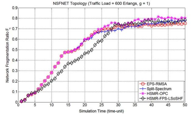
Fig. 8. Simulation results on network fragmentation ratio in NSFNET for HSMR schemes using traffic load at 600 Erlangs and  $g = 1$ .
