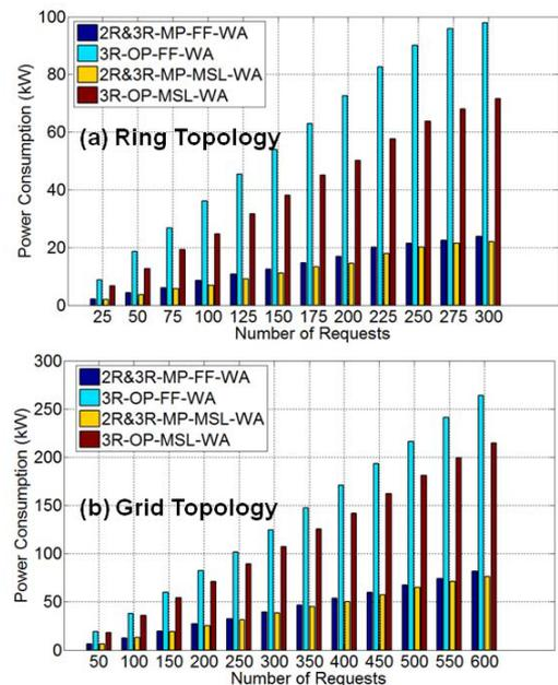
Fig. 3 Comparisons of power consumption in (a) a ring topology and (b) a grid topology ([15])
