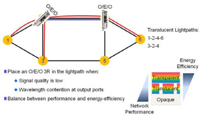
Fig. 1 An example of optical translucent network.
