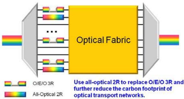
Fig. 2 Hybrid configuration of regeneration site.
