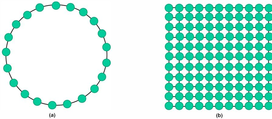
Fig. 2 (a) Ring network topology, (b) Grid network topology.
