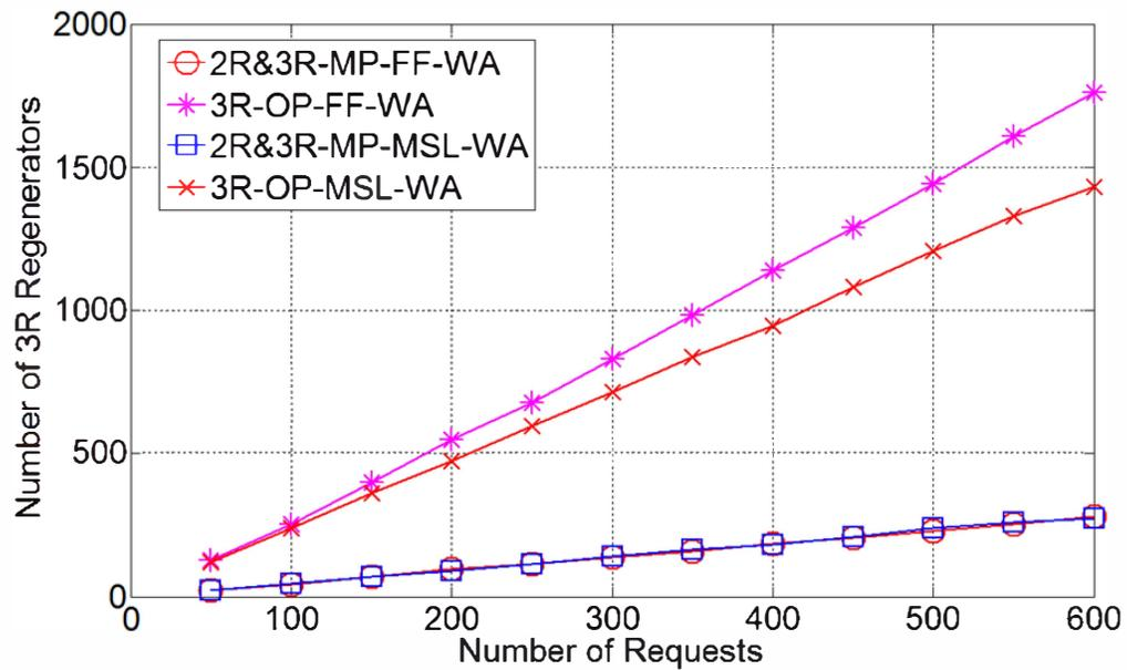
Fig. 5 Average number of 3R regenerators needed in grid network.
