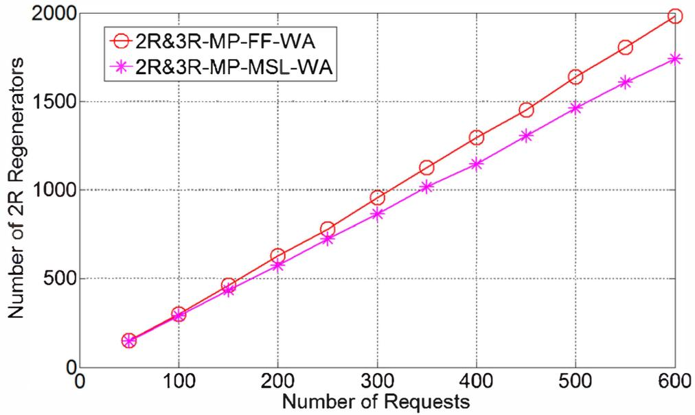
Fig. 6 Average number of 2R regenerators needed in grid network.
