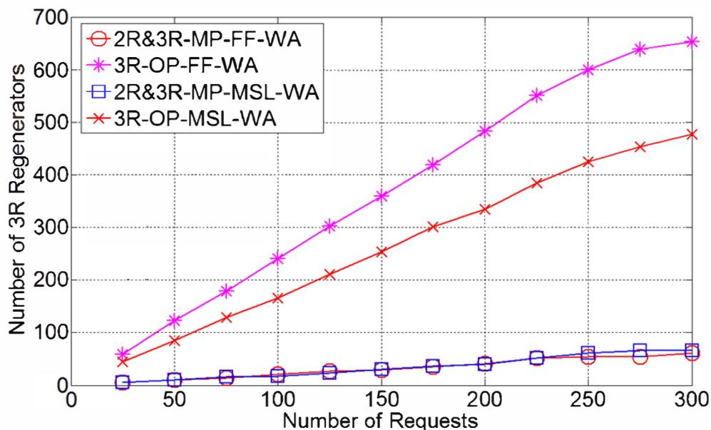
Fig. 3 Average number of 3R regenerators and needed in ring network.
