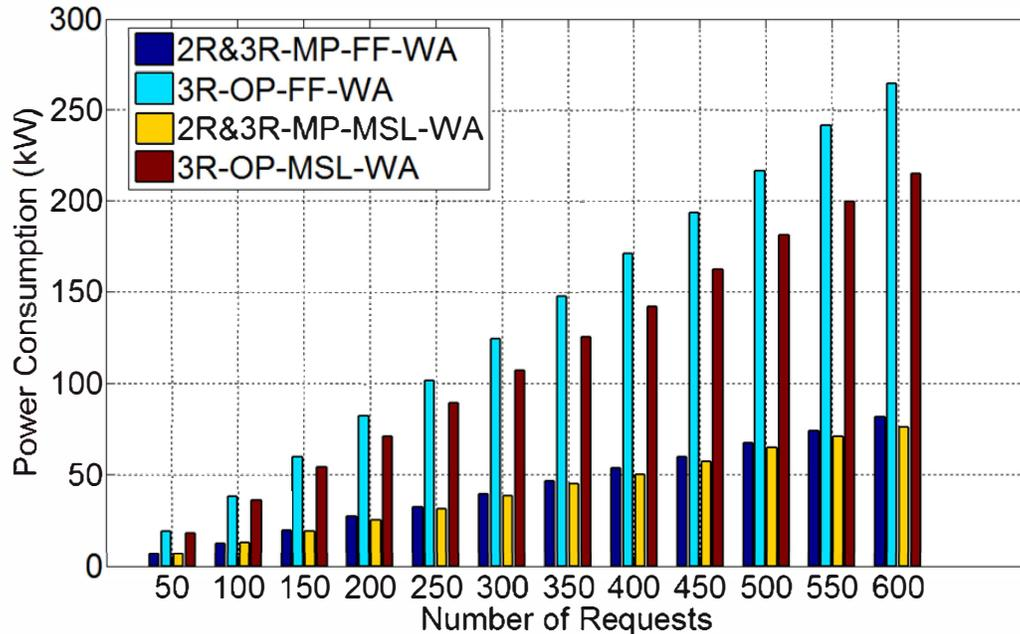
Fig. 8 Comparisons of regenerator power consumption for different design approaches in the grid network.
