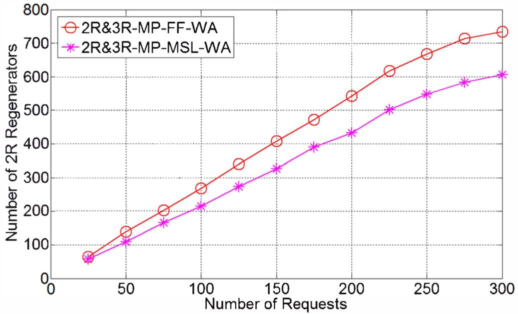
Fig. 4 Average number of 2R regenerators needed in ring network.
