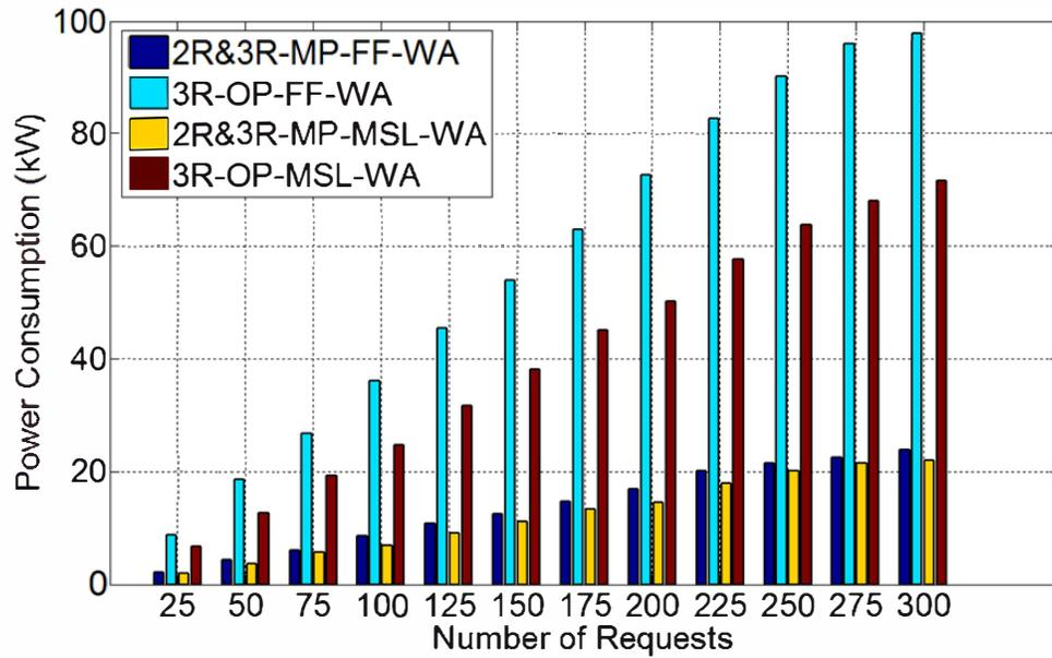
Fig. 7 Comparisons of regenerator power consumption for different design approaches in the ring network.
