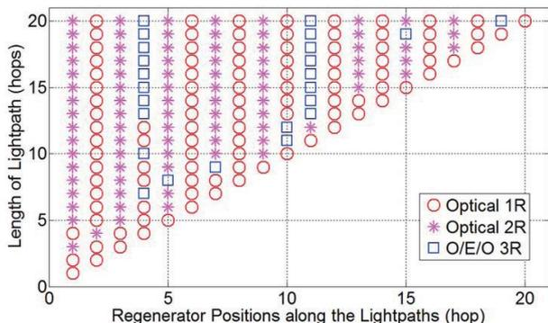
Fig. 5. 1R/2R/3R placements for lightpaths with random lengths.
