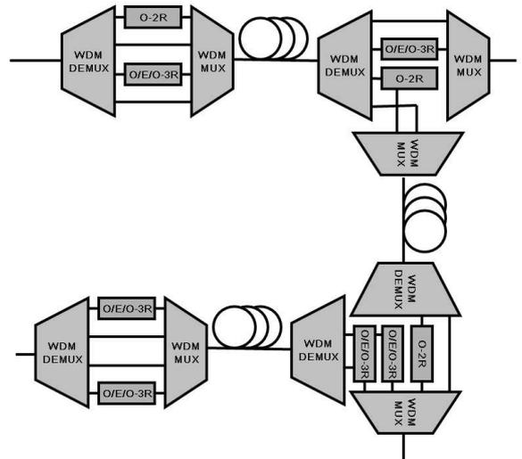
Fig. 1. Configurations of regeneration sites in our proposed translucent optical networks.
