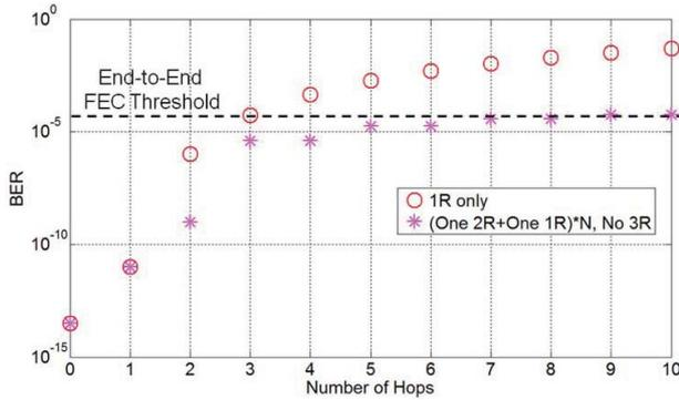
Fig. 3. End-to-end BER for lightpaths with different configurations.
