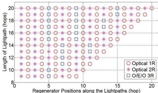
Fig. 4. 1R/2R/3R placements for lightpaths with lengths of 9 to 20 hops.
