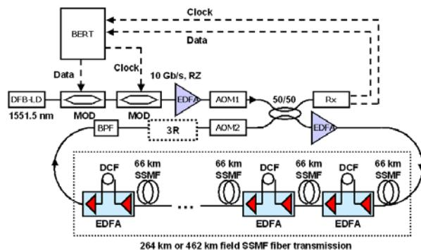
Fig. 2: Experimental setup, BERT: Bit-error-rate-tester, DFB-LD: DFB laser diode; MOD: LiNbO<sub>3</sub> modulator; AOM: Acoustic optical modulator; BPF: Optical band-pass filter; EDFA: Erbium-doped fiber amplifier; SSMF: Standard single-mode fiber; DCF: Dispersion compensating fiber; RX: Optical receiver
