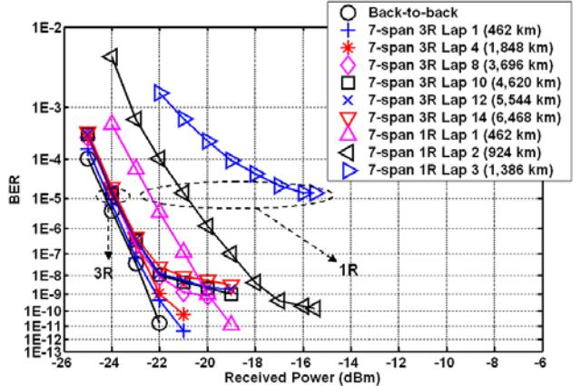
Fig. 7: BER measurement results of 462 km fiber recirculation loop experiments
