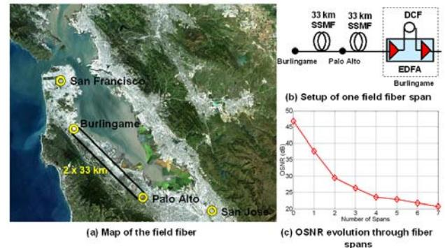
Fig. 1: (a) Map of the field fiber; (b) Setup of one field fiber span, SSMF: Standard Single-Mode Fiber, DCF: Dispersion Compensating Fiber, EDFA: Erbium-doped Fiber Amplifier; (c) OSNR evolution through field fiber spans
