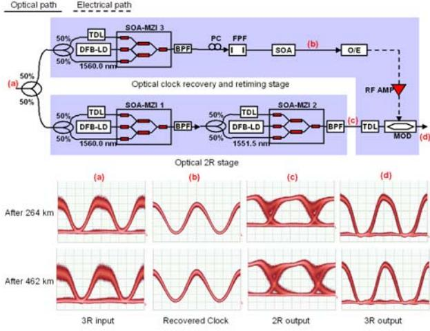
**Fig. 3:** All-optical 3R regenerator setup, TDL: Tunable delay line; DFB-LD: DFB laser diode; SOA-MZI: Semiconductor optical amplifier based Mach-Zehnder interferometer; BPF: Optical band-pass filter; PC: Polarization controller; FPF: Fabry-Perot filter; SOA: Semiconductor optical amplifier; O/E: Optical-to-electrical converter; RF AMP: RF amplifier; MOD:  $\text{LiNbO}_3$  modulator
