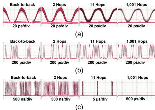
Fig. 2. (a) Eye diagrams, (b) bit patterns, and (c) packet sequences observed at OUT 2 for different hop counts.
