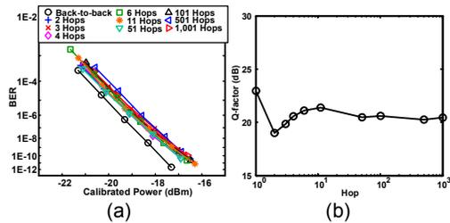
Fig. 3. (a) BER v.s. calibrated optical packet power. (b) Q-factor evolution for calibrated power of -12 dBm.
