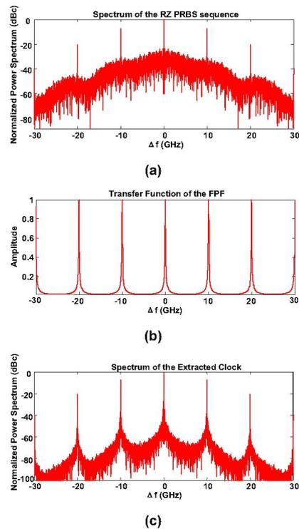
**Figure 1: Simulated spectra of clock recovery using FPF. (a) Spectrum of the RZ  $2^{23}-1$  PRBS at 10 Gb/s. (b) Transfer function of the FPF. (c) Spectrum of the extracted clock. The free spectrum range of the FPF is 10 GHz; the finesse is 100.  $\Delta f = 0$  represents the optical carrier frequency.**
