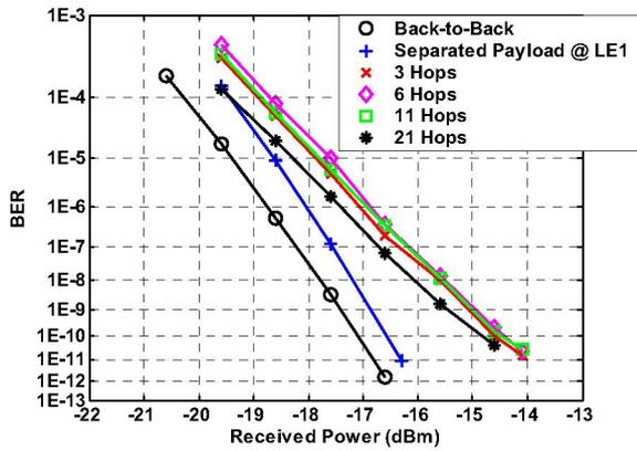
Figure 5: BER measurement results for OUT2.
