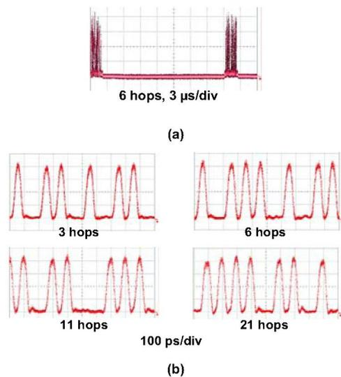
Figure 4: Oscilloscope traces observed at OUT2. (a) Packet sequence for 6 hops. (b) Bit pattern for 3, 6, 11, and 21 hops.
