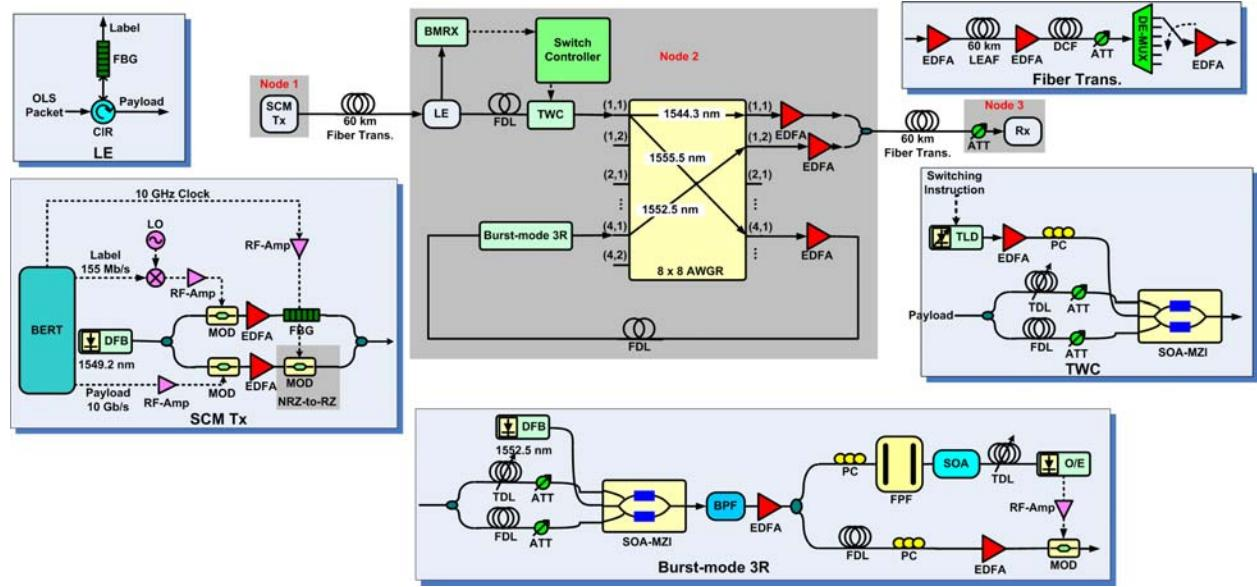
Fig. 2 Experimental Setup, BERT: Bit-error-tester, LO: Local oscillator, RF-amp: RF amplifier, EDFA: Erbium-doped fiber amplifier, CIR: Optical circulator, BMRX: Label burst-mode receiver, DE-MUX: De-multiplexer, PC: Polarization controller, TDL: Tunable delay line, FDL: Fixed delay line, BPF: Band-pass filter, O/E: Optical-to-electrical converter, Rx: optical receiver.
