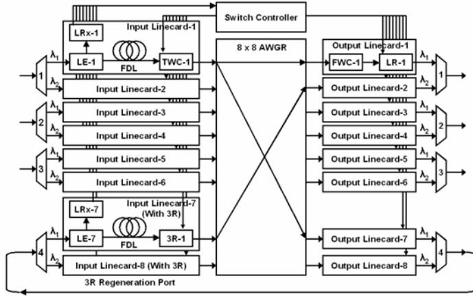
Fig. 1 Simplified architecture of an OLS router with limited 3R capability, LE: label extractor, LRx: label receiver, TWC: tunable wavelength converter, AWGR: arrayed waveguide grating router, FWC: fixed wavelength converter, LR: label rewriter.
