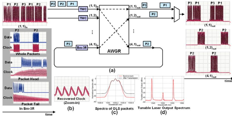
Fig. 3 (a) Timing diagram and the oscilloscope screens of the payloads, (b) Zoom-in screen of received burst-mode clock, (c) Spectra of OLS packets, (d) Tunable laser output spectrum
