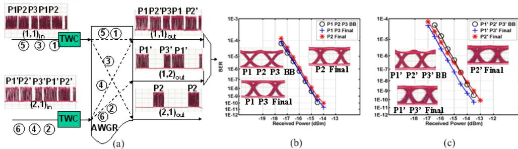
Figure 2 (a) Packet Sequence at the input and output ports (b) BER curves and eye diagrams for the P1 P2 P3 generated at Node 1 (c) BER curves and eye diagrams of the P1' P2' P3' generated at Node 2
