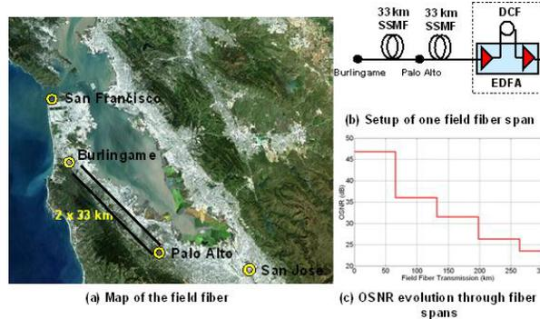
Figure 3 Characteristics of the field fiber plant (a) Map of the field fiber (b) setup of one of the field fiber span, SSMF: standard single-mode-fiber; DCF: dispersion compensated fiber; EDFA: Erbium doped fiber amplifier
