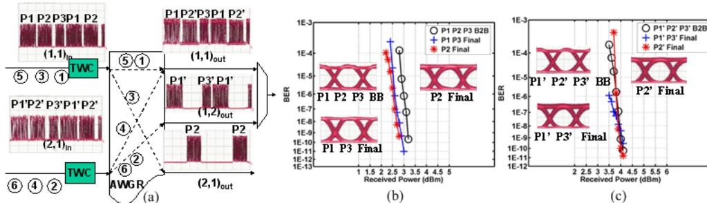
Figure 4 results of field trial experiment (a) packet sequence at the input and output ports (b) BER curves and eye diagrams of packets generated at Node 1 (c) BER curves and eye diagrams of packets generated at Node 2
