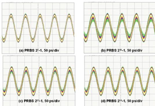
**Fig. 2 Clocks recovered from signals after 60 km fiber transmission with (a) PRBS  $2^7-1$ , (b) PRBS  $2^{15}-1$ , (c) PRBS  $2^{23}-1$ , and (d) PRBS  $2^{31}-1$**
