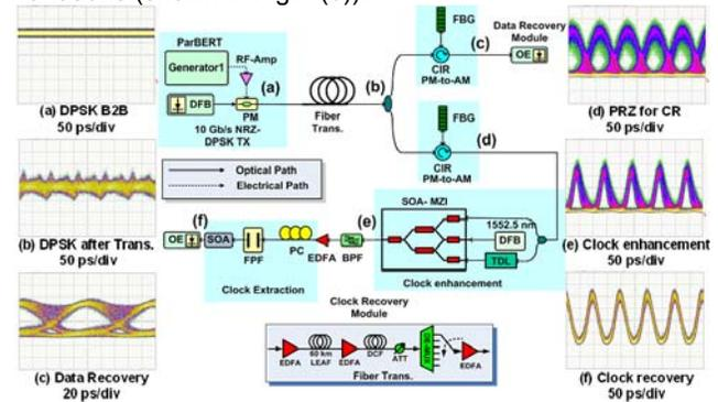
**Fig. 1 Experimental Setup, ParBERT: Parallel Bit-Error-Rate Tester, ATT: optical attenuator, BPF: optical band-pass filter, CIR: optical circulator, DFB: DFB laser diode, TDL: tunable delay line, OE: Optical to Electrical Converter, PM: phase modulator, PM-to-AM: phase modulation to amplitude modulation conversion, DEMUX: optical wavelength demultiplexer, (a)-(e) Eye diagrams measured at different locations as labeled in the setup**
