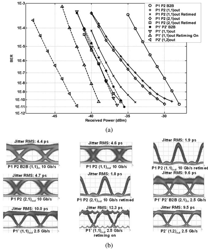
Fig. 3. Experimental results. (a) BER curves. Left: 10-Gb/s payload; right: 2.5-Gb/s payload. (b) Input and output payload eye diagrams. Time scale: 20 ps/div for 10 Gb/s and 100 ps/div for 2.5 Gb/s.
