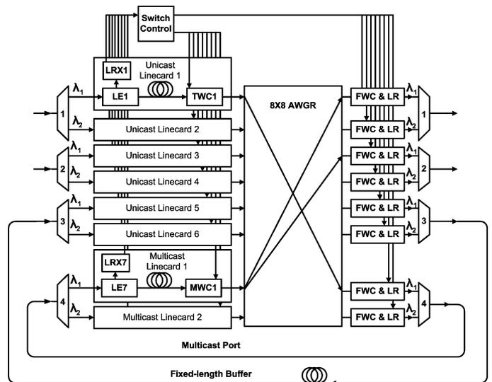
Fig. 1. Architecture of an OLS router supporting limited multicast function.
